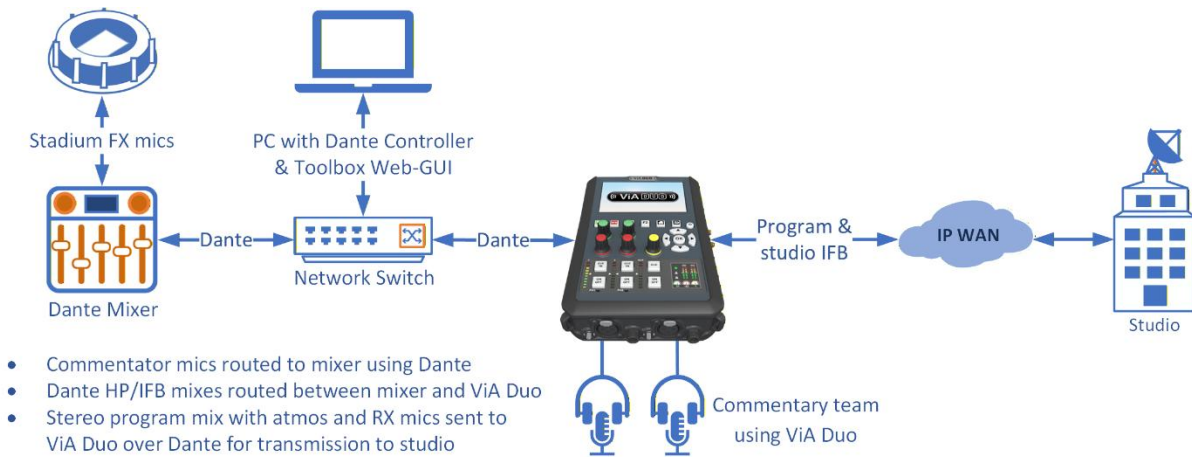
Remote radio commentary with integrated Dante devices
