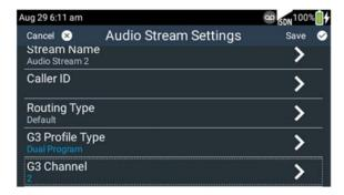
This ensures the correct encoder is used by the ViA when dialing IP1 and IP2 connections on a G3 codec.
