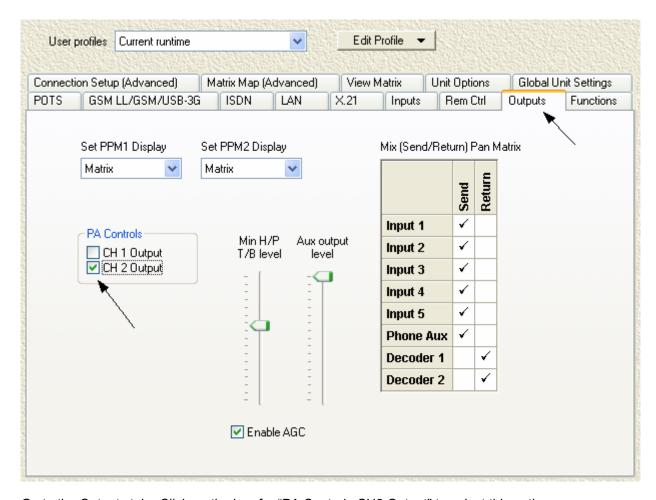
Go to the Outputs tab. Click on the box for "PA Controls CH2 Output" to select this option.
