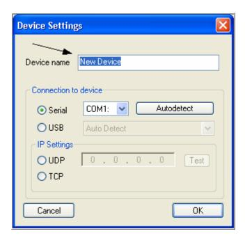
Enter a name for the new device (such as i-Mix G3) then click on the way you want to connect (such as USB).
