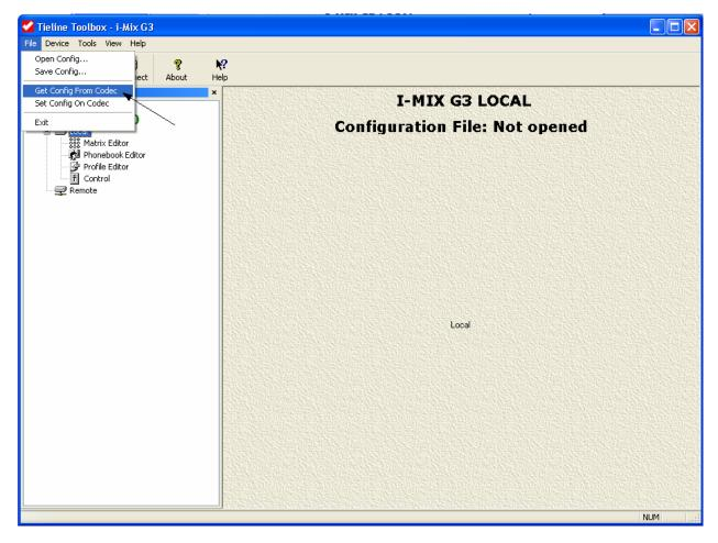
In the Tieline Toolbox software, select <u>Profile Editor</u> and then "Get Config From Codec" under the File pull down menu.
