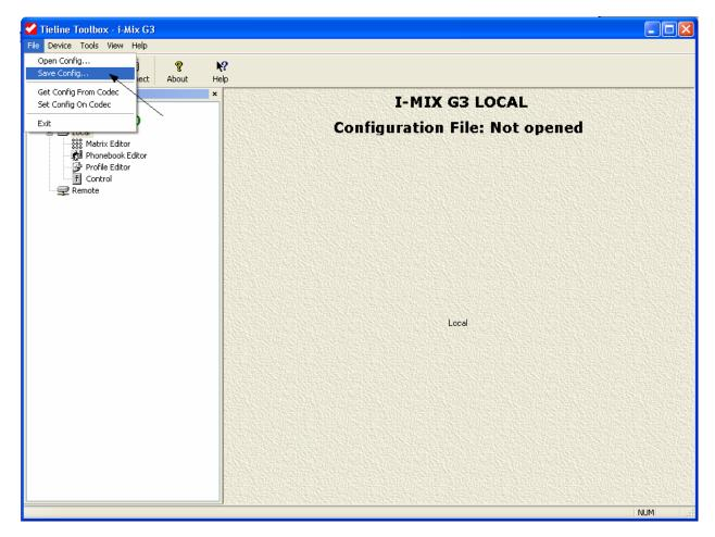
On the File pull down menu, select "Save Config" and save the original configuration to your PC (in case you need to reload the original configuration).
