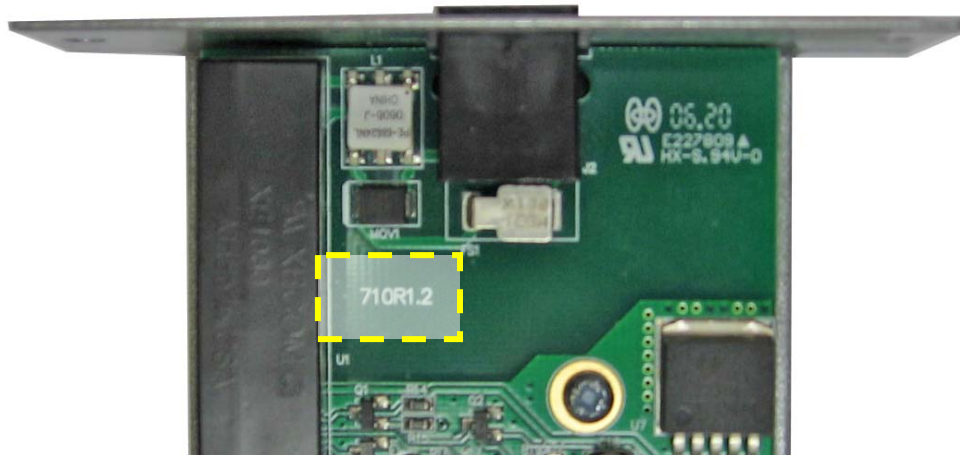
Figure 1: Voice-Capable Original POTS Module 710R1.2
