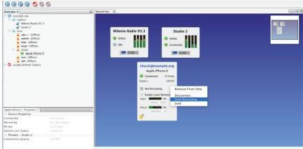
monitoring and remote control of all ViA, Merlin, Genie and Bridge-IT<sup>+</sup> codecs, as well as smartphones using Report- IT Enterprise.
