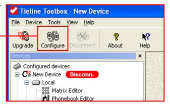
The codec is now able to communicate with ToolBox on the PC. The red disconnected (*Disconn.*) device goes to a green *Connected* mode. You can change the settings on your codec and any remote units to which your local codec is connected via ToolBox software.
