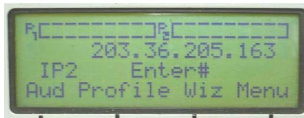
6. Press the **ENTER DIAL** button on the codec's grey keypad to dial and connect using the connection profile you have selected, e.g. mono, stereo, mono/IFB or dual mono. Note: In most situations it is only possible to dial from the remote codec to the studio codec over IP because only the studio codec is using a public IP address.
