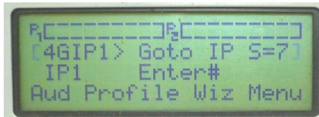
5. Next scroll to **IP1** on the main codec LCD screen and type the IP address of the codec you are dialing. (Note: Use the \* or # button on the codec keypad to enter the periods (.) in the IP address).
